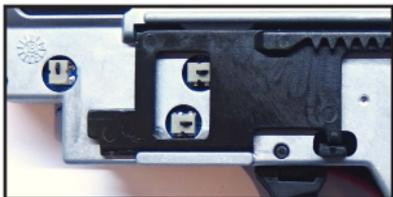
4. Check other side if all 3 micro switches are in the center of the holes.
