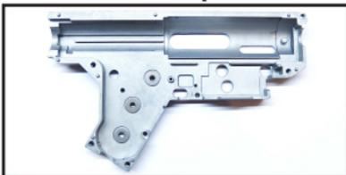
1. Prepared gearbox for installation.
