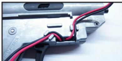
**13.** Insert all internals into the gearbox, screw gearbox together and place wires to the holders on the picture.
