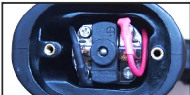
**18.** Connect wires to the motor. Keep in mind right motor polarity.
