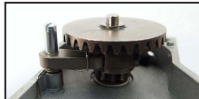
4. Use glue to hold screw in place. Test if ARL holds gear to not spin clockwise. ARL mode is finished now. 2
