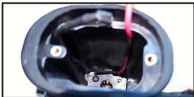
**16.** Black wire bends back at the bottom of the grip and red wire lead to the front.
