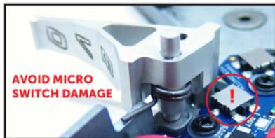
5. Carefully insert the trigger into the gearbox in rest position. Trigger spring must be outside the gearbox.
